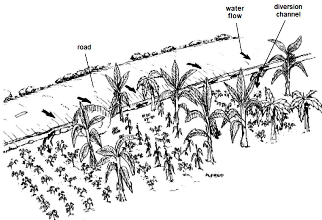
FIGURE 5-6 - RAINWATER HARVESTING USING A ROAD CATCHMENT
